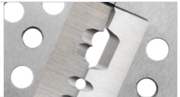
Two pairs of blades (1) cut the insulation to complete extent. Then the blade pairs move apart, and thus the insulation is removed form-fit (2). The pliers opens automatically after the stripping procedure.
