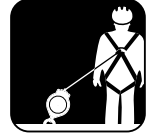
* It can be used where the Anchorage point is available at foot Level also.
